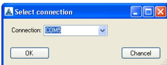
All currently available COM ports are displayed in the list (which can be opened with the downward arrow). INDULVENT ec generally has the port with the highest number. The COM port should be selected and the selection should be confirmed with "OK."
