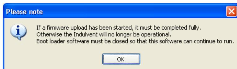
Clicking the "OK" button does not start an upload; the upload is started in the program that opens. The control system is thus still running after "OK" is clicked.
