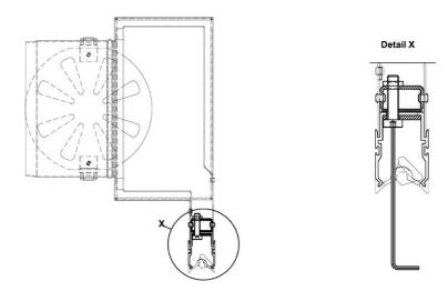
The INDUL AV24, AV124, AV45 and AV145 models can be supplied with a separable connection between the support profile and the plenum box, so that the plenum is cleanable according to VDI 6022. The separable connection is not possible in combination with integral or loose plaster brackets...NG.
