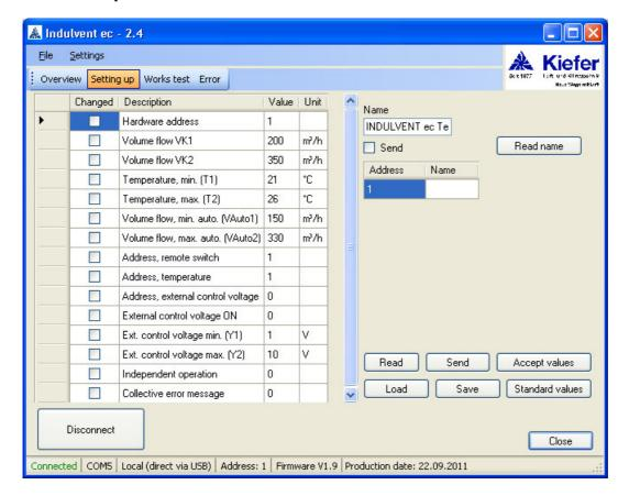
The respective parameters can be adapted in the Value column. If a minimum value is not achieved or a maximum value is exceeded in the process, the values are limited to the minimum or maximum value. A plausibility check does not take place. Larger values may be entered for a minimum value than for the maximum value. This could lead to malfunctions in INDULVENT ec, however.
