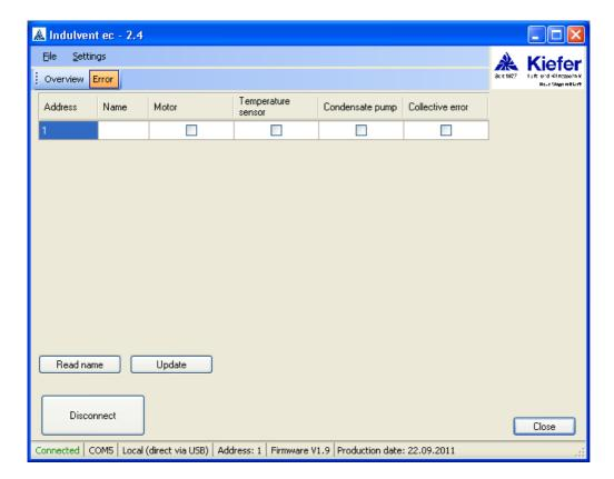
All connected INDULVENT ec devices and their respective statuses are included in the list. In case of a check mark by "Motor," "Temperature sensor", "Condensate pump", or "Collective fault message", the respective location has a fault.
