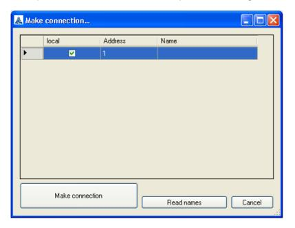
All devices connected to the bus are shown here. Using the "Read Names" button, the names of all bus subscribers can be read.
