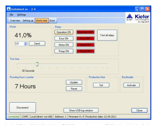
In the "Pulse Width Modulation (PWM)" area, the current PWM with which the fan is actuated is displayed. The PWM can be changed by entering the corresponding value and clicking "Send". The PWM value can be set between 0 and 100%.
