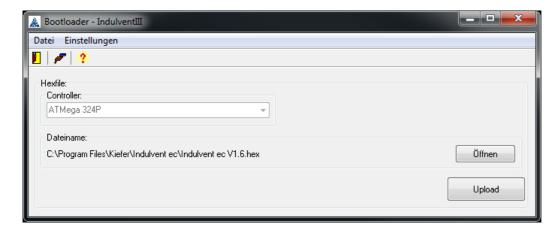
The firmware upload is started by clicking the "Upload" button.
