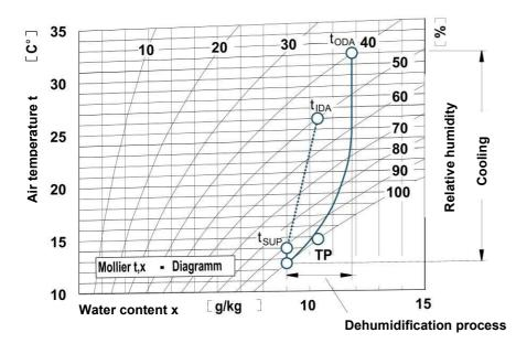
t<sub>ODA</sub> = Outdoor air temperature t<sub>IDA</sub> = Measured ambient air temperature t<sub>SUP</sub> = Supply air temperature TP = Dew point
